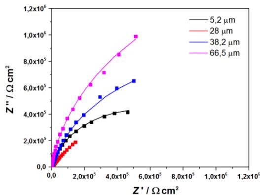
Nyquist plot (EIS) after potentiostatic polarization at 0.4 V<sub>Ag/AgCl</sub> for 6 hours. The semi-circle size indicates the charge transfer resistance that decreases with PAGS refinement up to a critical value while further refinement leads to an increase
