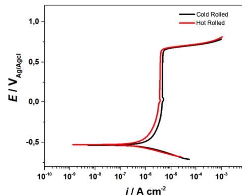
Potentiodynamic polarization curves of cold rolled and hot rolled IF steels, showing slightly higher passivity current density with increase in dislocation
