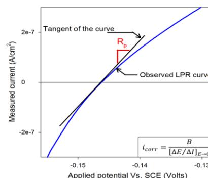
**Fig 1.** Extraction of the LPR value from the I-V curve.
