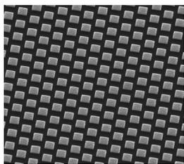
Electron microscope image of a microstructured diamond surface as grown in the lab of Buijnsters at TU Delft. Here, synthetic diamond layers can be produced with a structure already defined during growth, such that expensive lithographic and etching techniques are not necessary.
