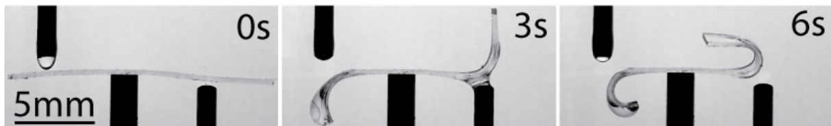
Figure 1: Self-folding of an elastomer by localized swelling [1]
