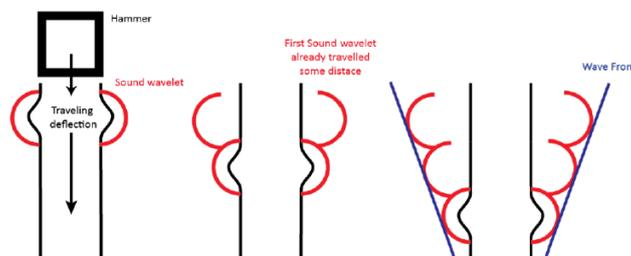
**Wave front radiation from offshore driven piles**
