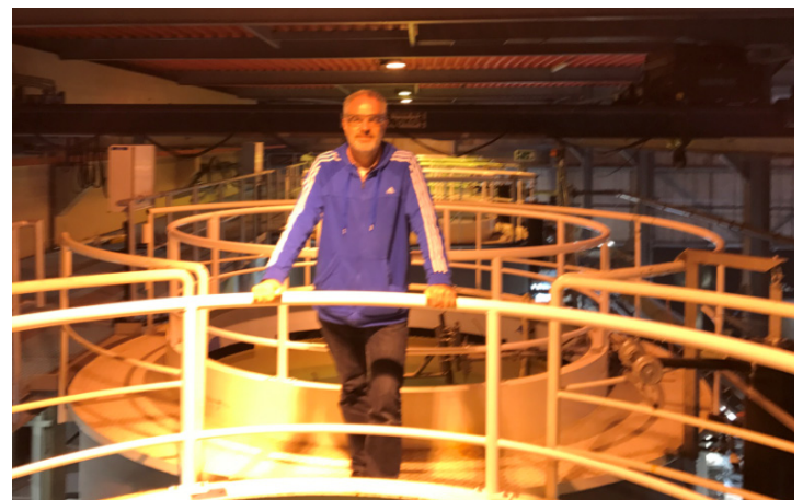
Figure 6 Full-scale pellet softeners at Waternet. Yearly, more than 400 million m^3 water is softened in the Netherlands.
