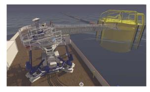
interaction between the Ampelmann system and the CALM buoy has been studied by a numeric, coupled, time-domain model. Using this model the response of the coupled system will be compared with and without the dynamic interaction of the gangway forces acting on the buoy.
