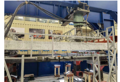
Continuous supported slab
