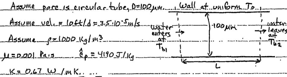
What is  $L$  for  $\frac{T_{o2} - T_{b2}}{T_{o1} - T_{b1}} = 0.01$ ? (99% of way to equilibrium)
