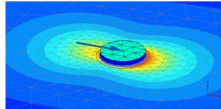
Soil Displacement along load direction (P = 30,000 kN)
