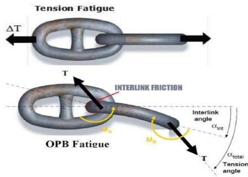
In 2002, several mooring chains of Girassol off-loading buoy which was installed offshore Angola, ruptured just after 8 months of service. After a series of investigations, a new failure mechanism called Out-Of Plane Bending (OPB) fatigue was identified. This failure mechanism is not considered in conventional assessment standards.
