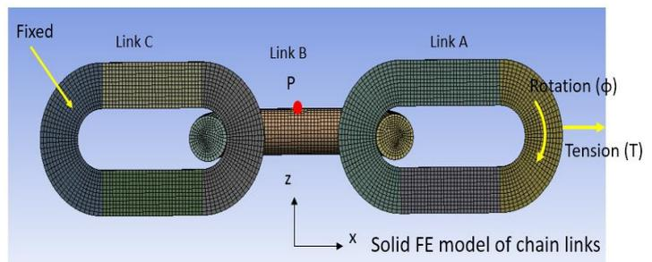
In this thesis, a new interlink stiffness model is proposed to describe the nonlinear hysteretic relationship between OPB moment/stress and interlink angle. The interlink stiffness model is then applied to a system of chain links using two different approaches: a physics based approach and a semi-empirical approach.
