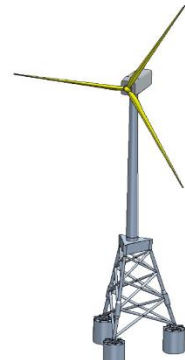
Suction Installed Wind Turbine
