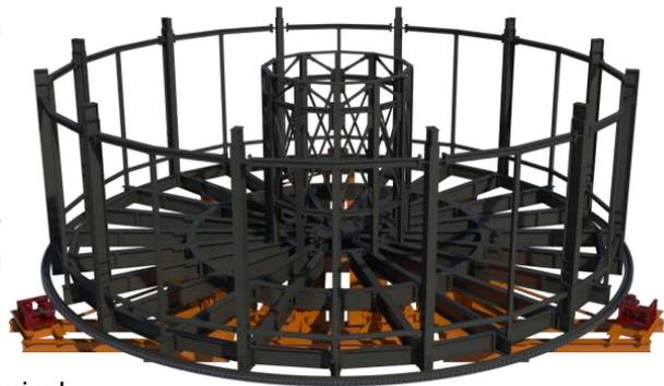
An experimental and analytical approach is used to obtain a better understanding of the mechanical behaviour. A scale model is built to gain knowledge about the physical behaviour of cable, obtain a distribution of forces on the basket walls and obtain hands-on experience. The experiments can also be used to improve and validate theoretical models.
