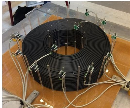
Three experiments were performed: static wall deflection test, acceleration test and the (in)-stability test. The wall deflection test is used to determine the static deflection of the walls due to the cable. The acceleration test is used to determine the dynamic influence of the cable loads on the walls. The (in)-stability test is done to show a relation between the acceleration and stability of the cable package.
