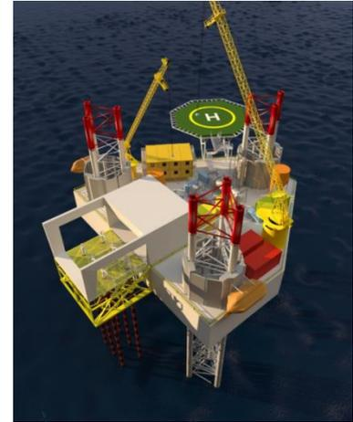
Due to low oil and gas prices since 2015 the occupation of jack-up drilling rigs has declined. Some of these idle rigs are in line to be scrapped and could be potentially acquired for a low price. The idea was suggested within ONE to convert an idle drilling rig into a production platform.
