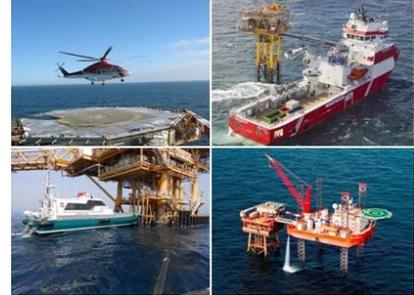
The access of an offshore structure can be obtained in different ways. TEPNL's current operating mode for accessing her structures is a combination of: helicopter to transport people and a supply vessel to transport materials. The personnel transfer from a vessel to an offshore structure is called marine access. TEPNL is interested to know if any form of marine access could help to optimize offshore operations and this is the topic of this MSc thesis.
