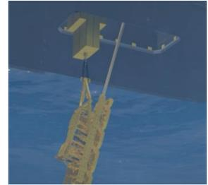
The installation analysis of the 18" ILT-structure installations involved in the Ichthys project shows high compression in the upper- and upper-counter stem, the connection between the ILT and the pipe. Although Flexcom shows that buckling limits are exceeded, offshore load measurements of previous installations show hardly any compression.
