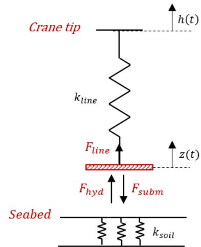
The hydrodynamic or added mass force acting on the disk is similar to the method described in literature by Brennen. Brennen's flat plate analogy has been applied and used to derive a force acting on a closed disk (1D model) and one for an open disk (2D model). Whereas the 1D model includes only horizontal fluid flow velocity, the 2D model also takes vertical flow velocity into account.
