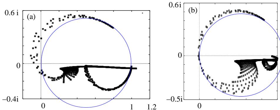
Figure 6: Spectral pictures of preconditioned system with one two-grid iteration used for preconditioning  $(\beta_1, \beta_2) = (1, 0.5)$ ,  $k = 40$ ,  $h = 1/64$ , (a) one  $\omega$ -JAC relaxation, (b) two  $\omega$ -JAC relaxations,  $\omega = 0.5$  (the eigenvalues with exact inversion lie at the circles).
