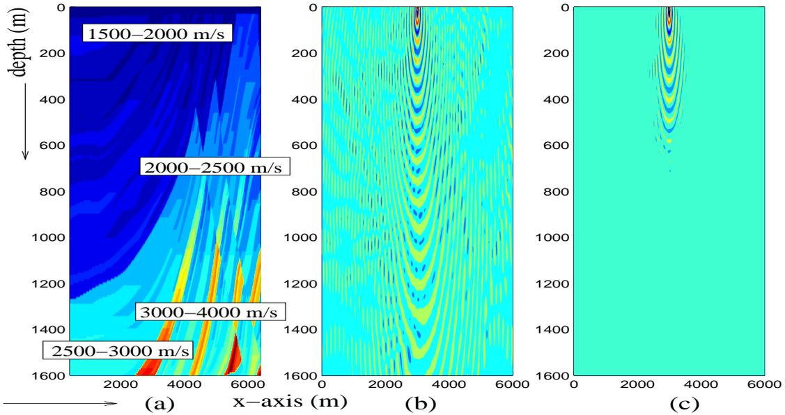
Figure 10: Marmousi problem (not to scale). a) Velocity distribution in meter/s, b) real part of the solution for  $f = 20$  Hz, no damping, c) real part of the solution for  $f = 20$  Hz, 2.5 % damping.
