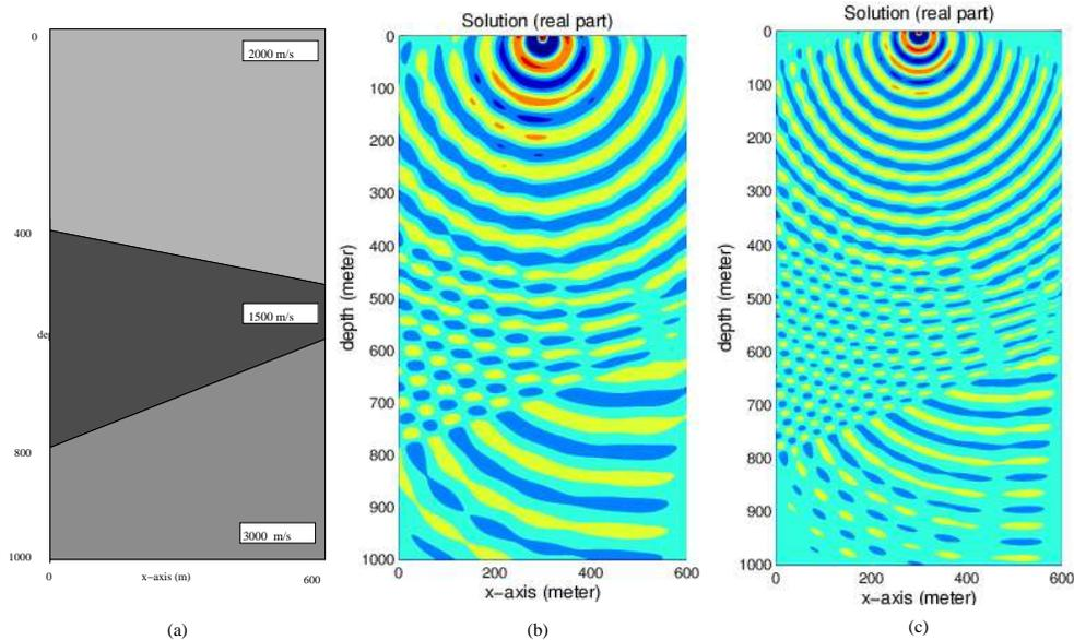
Figure 8: Wedge problem: (a) Problem geometry with velocity profile indicated, (b) Real part of numerical solution at 30 Hz, (c) Real part of numerical solution at 50 Hz.
