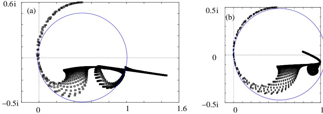
Figure 5: Spectral pictures of preconditioned system with one two-grid iteration used for preconditioning  $(\beta_1, \beta_2) = (1, 1)$ ,  $k = 40, h = 1/64$ , (a) one  $\omega$ -JAC relaxation, (b) two  $\omega$ -JAC relaxations,  $\omega = 0.7$  (the eigenvalues with the exact inversion lie at the circles).
