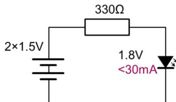
The source must supply at least 1.8V → the lowest number is  $2 \times 1.5V = 3V$ . The excess  $3 - 1.8 = 1.2V$  must be dissipated by a resistance. The maximum current is 30mA → all resistors are acceptable. For the chosen  $R = 330\Omega$ ,  $I = 1.2/330 = 3.6mA$  and  $P_{dissipated} = 1.2^2/330 = 4.4mW$ .
