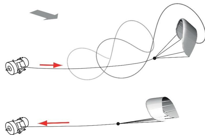
In the reel-out phase the kite flies in figure eight patterns capturing crosswind energy.
