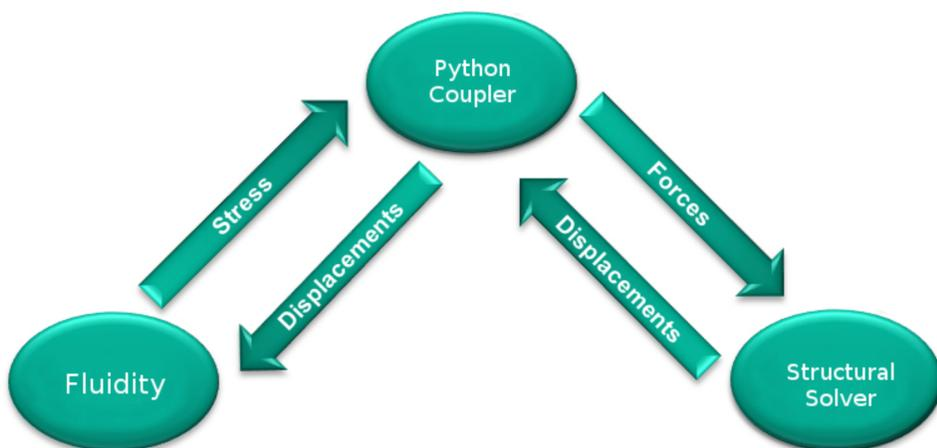
**Stage 1:** Fluidity [3] coupled with an in-house structural solver on membrane elements.
