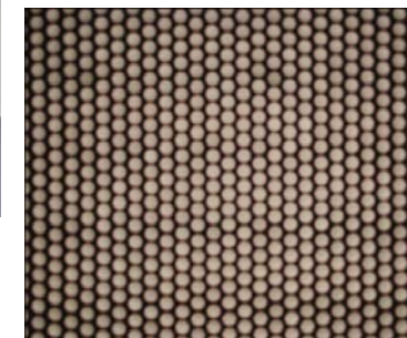
Acoustic damping holes drilling
