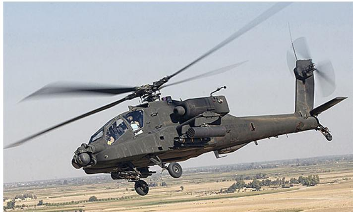
Helicopter pilots use the rotors to move their aircraft upwards and downwards and to steer them sideways. With a stick they are able to adjust the angle of the rotors, which causes the helicopter to move to the left or the right and forward or backward. But when performing these maneuvers in forward flight helicopters can experience large and sometimes even unacceptable loads on the main rotor system.
