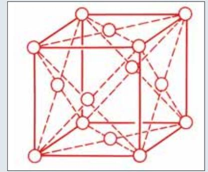
Crystal structure of austenite in pure iron. Austenite is stable at temperatures over 912 °C. The iron atoms are arranged in a regular pattern at the vertices and in the centres of the six surfaces of an imaginary cube. The structure is known as face-centred cubic.
