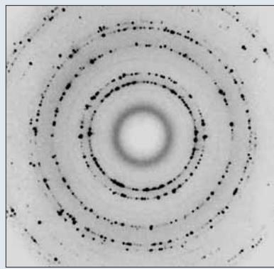
Diffraction pattern of austenite. At temperatures around 900 °C, austenite is the stable phase in the carbon steel used. The dots on the detector are all the result of the diffraction of the X-rays by individual austenite crystals within the steel sample. The size of an individual crystal can be deduced from the intensity of the dots, since a large crystal will diffract more X-rays and thus produce a higher intensity.
