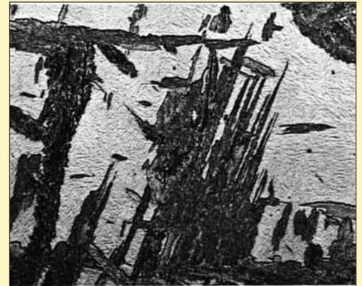
Optical microscope image of bainite (dark areas) at room temperature. Like pearlite, bainite is a composite of ferrite and cementite, but it has a totally different microstructure. Bainite consists of ferrite needles interspersed with cementite.
