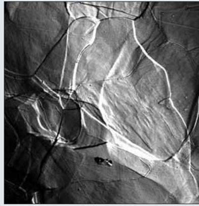
Microscope view of austenite in pure iron. The image was obtained using a laser-scanning confocal microscope at a temperature of 1000 °C.
