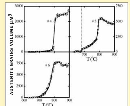
The disappearance of individual austenite crystals. Inevitably, the growth of ferrite causes the disappearance of austenite crystals. Within the disappearing austenite, although the first three types of ferrite growth (see previous illustration) can be detected, the fourth type cannot. The disappearance of the austenite leads to the conclusion that carbon atoms are being exchanged between different austenite crystals.
