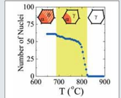
The number of ferrite nuclei measured in carbon steel that was cooled in one hour from 900 °C down to 600 °C. Offerman's measurements show that the activation energy required to produce ferrite crystals is at least a hundred times less than previously assumed. This knowledge is of crucial importance for modelling phase transformations in steel.
