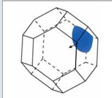
Schematic diagram of an austenite crystal with a ferrite crystal growing inside it. By preference, the crystal will start to grow on one of the corners of the austenite crystal, since that is the optimum location energy-wise.
