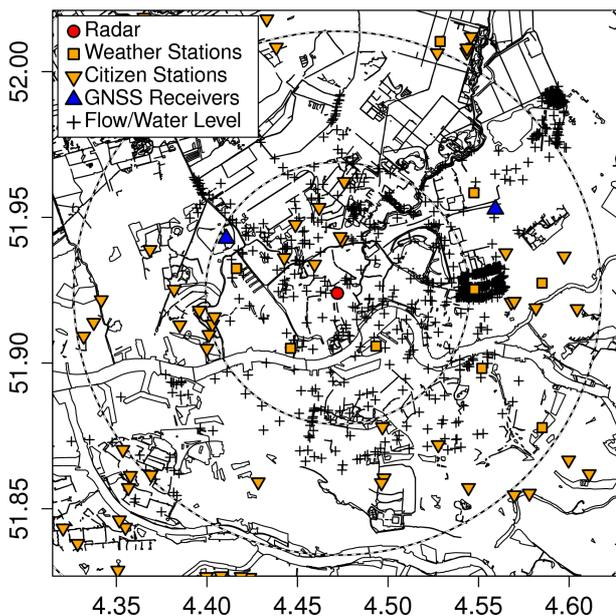
Map of sensors deployed within 10 km from the city centre of Rotterdam. In addition to the radar, there are about 50 citizen rain gauges and 10 professional weather stations. More information about the MUFFIN campaign can be found at [www.muffin-project.eu](http://www.muffin-project.eu).
