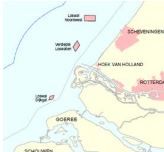
Figure 6. Relocation areas for dredged material (from Ebbens, 2013). The PoR uses only Verdiepte Loswal and Loswal Noord West for maintenance dredging.
