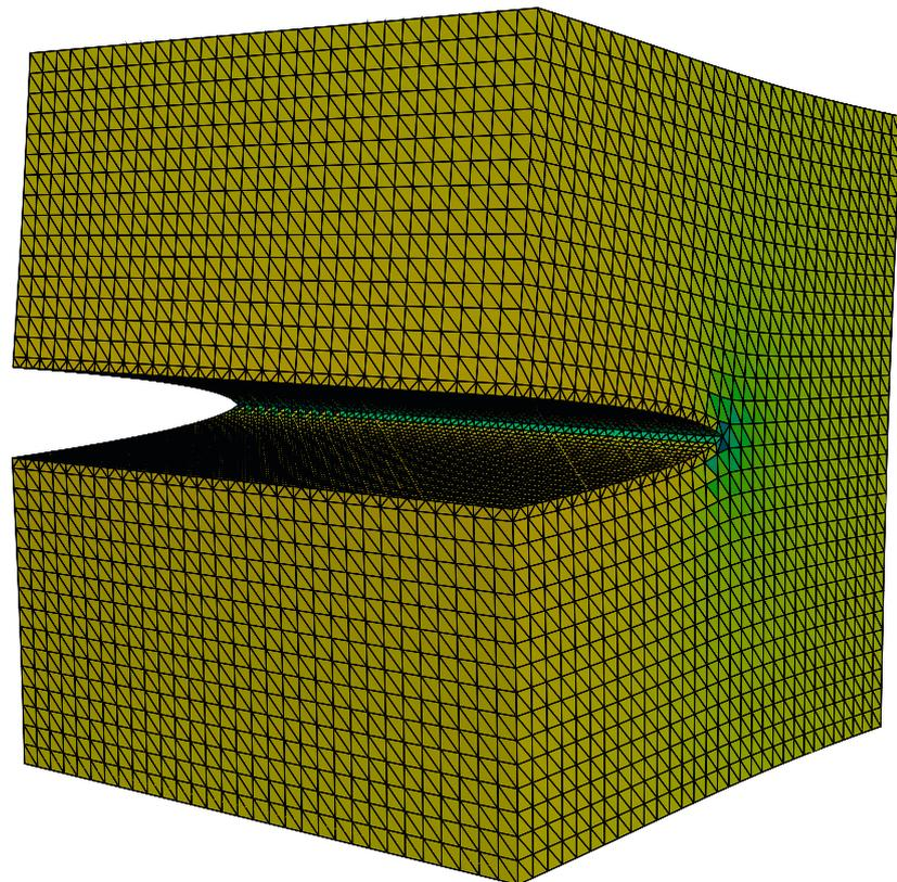
*Mode I opening of a cracked cube. What is remarkable about this simulation is that the crack was placed completely independently from the finite element mesh used: the latter was a simple structured mesh. So in order to see the displacement some post-processing is needed. This was carried out using Aragón’s Discontinuity-Enriched Finite Element Method.*
